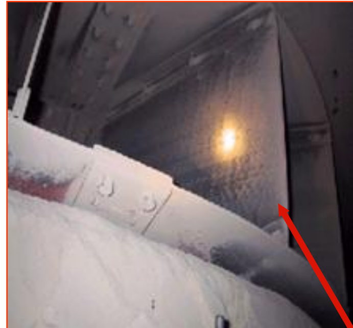
Fan blades Erosive wear HARDOX 500
